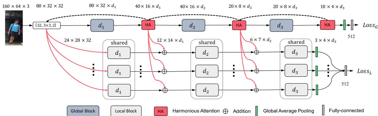
**Fig. 1** Schematic architecture of the proposed harmonious attention network (HAN). The design of HAN is characterised by high cost-effectiveness for maximising the model scalability. This is enabled by the introduction of a lightweight but effective harmonious attention
