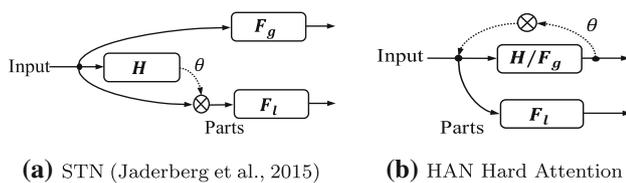
**Fig. 3** Schematic comparison between **a** spatial transformer network (STN) (Jaderberg et al. 2015) and **b** HAN hard attention. Global feature and hard attention are jointly learned in a multi-task design. “ $H$ ”: Hard attention module; “ $F_g$ ”: Global feature module; “ $F_l$ ”: Local feature module
