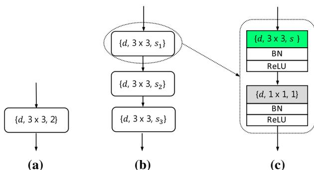
**Fig. 4** Structure of **a** local block and **b** global block. Each block **c** consists of two conv layers. Layer type is indicated by background colour: grey for *normal conv*, and green for *depthwise separable conv* layers. The three items in the bracket of a conv layer are: filter number, filter shape, and stride
