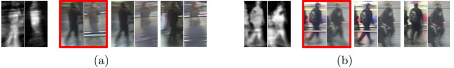
Fig. 6. (a) and (b) show two examples of the GEI gait features and our video fragment pairs. In both (a) and (b), the leftmost thumbnail shows GEI gait features, while the remaining thumbnails present some examples of fragment pairs, with the automatically selected pairs marked by red bounding boxes. A fragment is visualized as the weighted average of all its frames with emphasis on its central frame.
